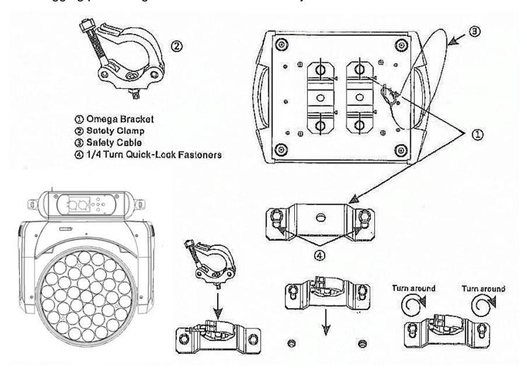
Regardless of the rigging option you choose for your B eye par, always be sure to secure your fixture with a safety cable. The fixture provides a built-in rigging point for a safety cable on the hanging bracket as illustrated above. Be sure to only use the designated rigging point for the safety cable and never secure a safety cable to a carrying handle.
