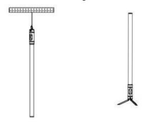
Equipped with removable ring, can be lifted useing removable triangle folding bracket, can be placed on the ground
